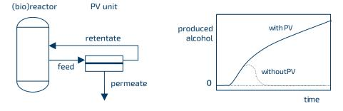
The image shows the principle of a membrane reactor for continuous product recovery (alcohols, aromas). The system with pervaporation continuously produces alcohol while other systems stop when inhibiting amounts of alcohol (or another inhibitor) have been reached. In some cases, a pretreatment is necessary. PDMS membranes are stable and insensitive to fouling.
