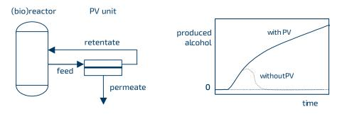
The image shows the principle of a membrane reactor for continuous product recovery (alcohols, aromas). The system with pervaporation continuously produces alcohol while other systems stop when inhibiting amounts of alcohol (or another inhibitor) have been reached. In some cases, a pretreatment is necessary.
