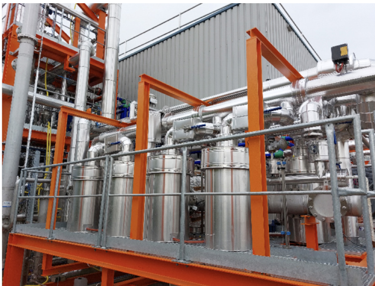
Figure 11: Industrial vapor permeation plant for IPA dehydration with PERVATECH Hybrid Silica HybSi® Acid Resistant membranes
